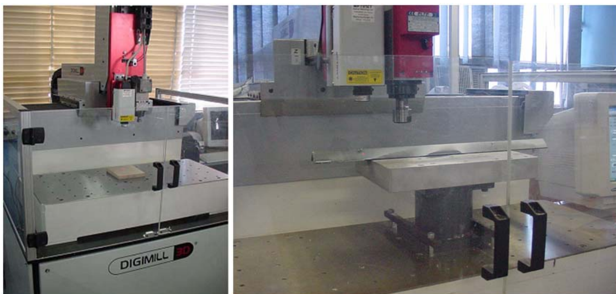
Figure 2: Three-dimensional laser scanner, Digimill 3D model, and studied L profile being scanned.
