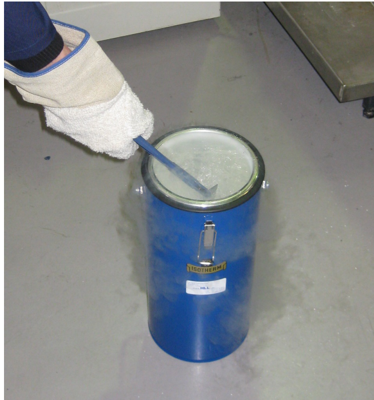
Figure 1. Cooling of specimen in a Dewar vessel filled with liquid nitrogen.
