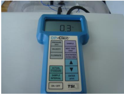
Figure 4. DP - Calc manometer used to measure static and total pressure
