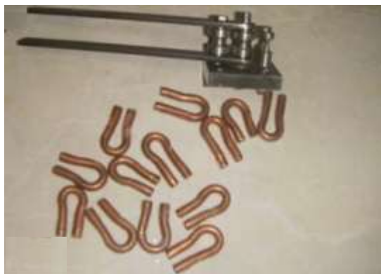
Figure 5. Connections to be welded in pipe extremities
