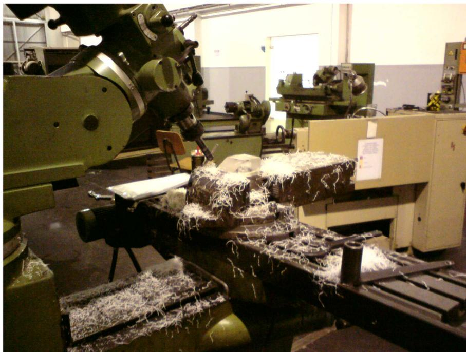
Figure 3 – Milling operation of the prostheses fixation platform.
