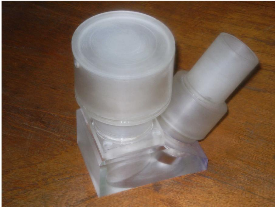
Figure 4 – Both aortic root and atrium model assembled at the prostheses fixation platform. Arrangement: aortic root upon the platform inclined plan, atrium model at the higher left position.
