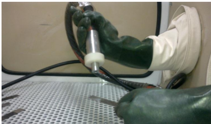
Figure 4. Blasting process with steel grit
