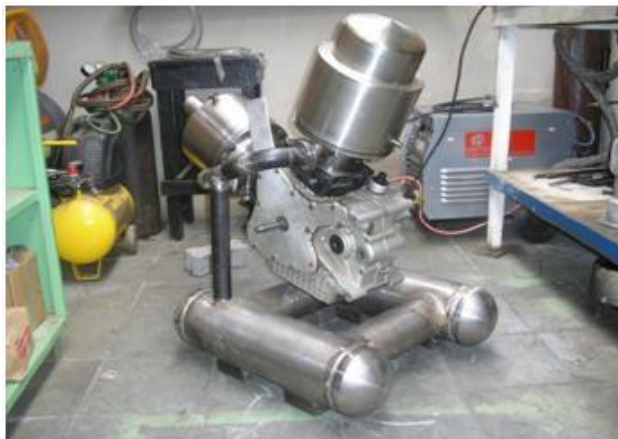
Figure 1. Simplified general scheme for the adaptations required by the Ducati engine block to operate as a Stirling engine of 8 kW power.
