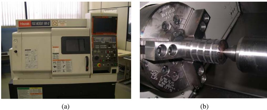
Figure 7. CNC lathe used for the experiments: (a) Mazak QTN 100-II; (b) workpiece to perform the operation
