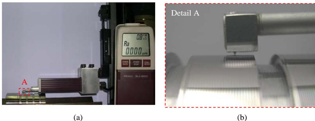
Figure 8. Roughness measurement system: (a) Mitutoyo roughness tester SJ-201; (b) Detail of probe in operation (13 $\times$ )
