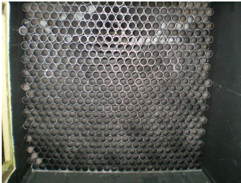
Figure 7. Box of uniformization of the type beehive.
