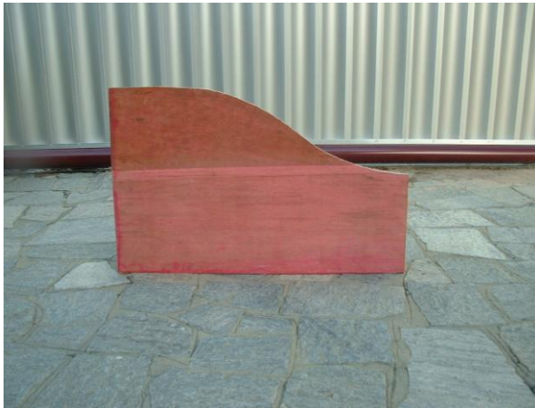
Figure 1. Molds for the diffuser.
