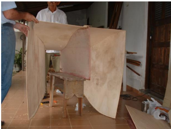
Figure 3. Assembly of the contraction.
