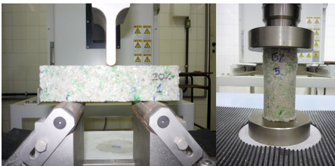
Figure 1. Flexural and compressive test set-up
