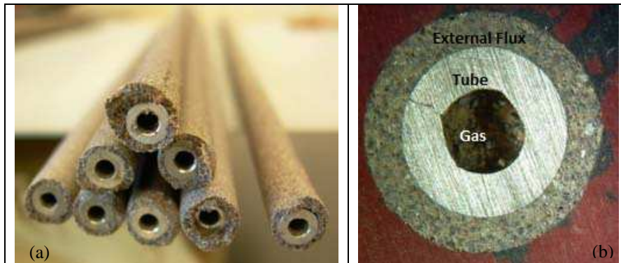
Figure 4. a) Tubular electrodes and, b) Cross section of a tubular electrode
