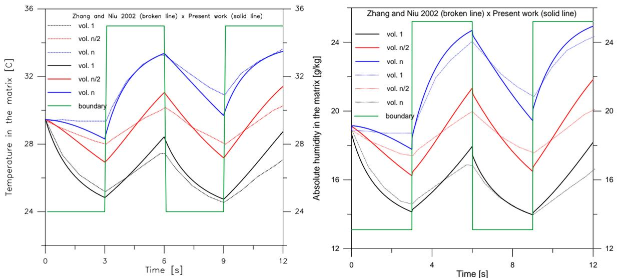
Figure 6. Temperature and absolute humidity into the desiccant matrix:
