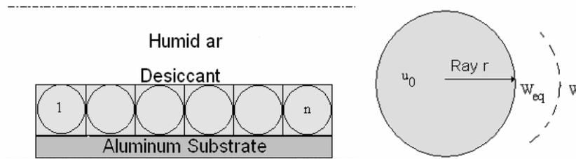
Figure 2. Schematic view of the enthalpy wheel and side view of one grain
