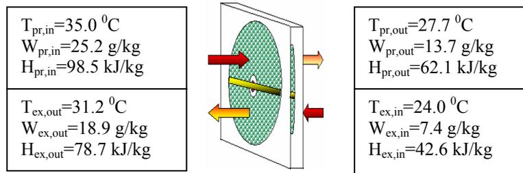
Figure 3. Hot test in the enthalpy wheel
