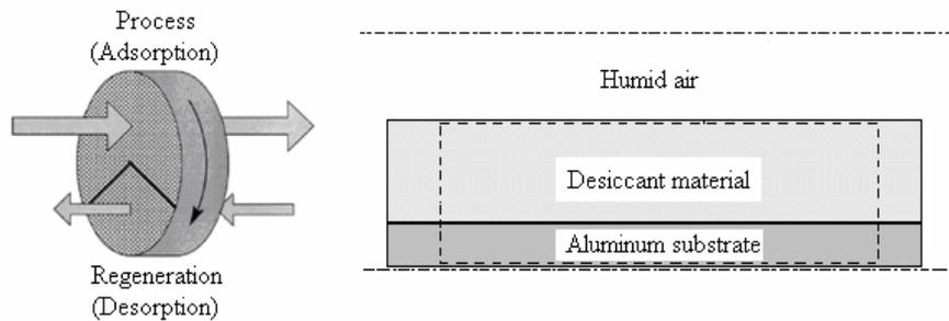
Figure 1. Schematic view of the enthalpy wheel and side view of one channel
