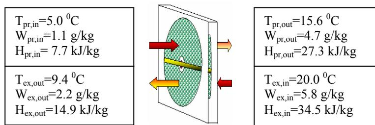
Figure 4. Cold test in the enthalpy wheel
