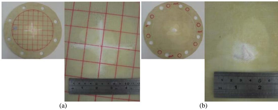
Figure 4: Rigid sphere impact against plate Fg05-32: (a) top view; (b) bottom view.
