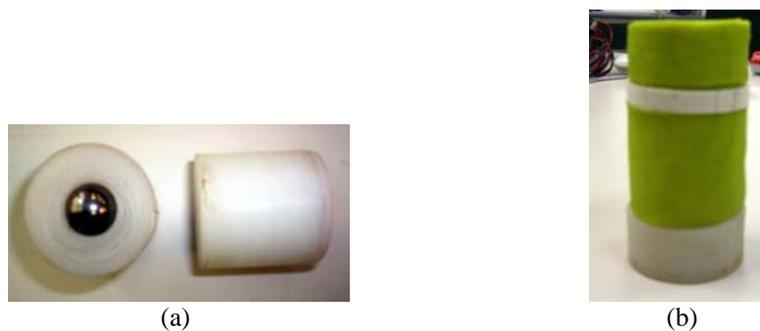
Figure 3: Projectiles employed in the tests: (a) Rigid sphere next to sabot; (b) Modeling compound cylinder.
