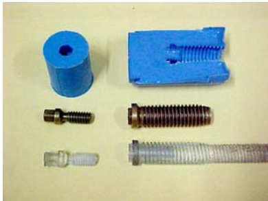
Figure 10 – Molds, implant and photoelastic sets generated.
