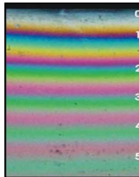
Figure 2. Isocromatic fringe orders.
