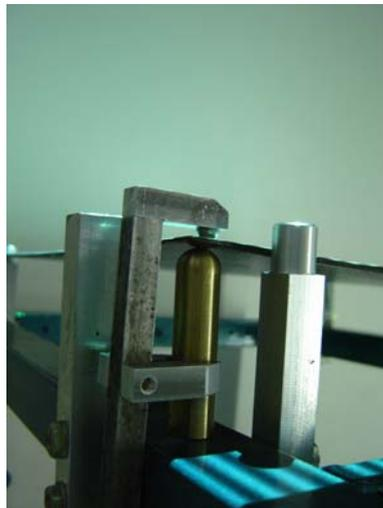
Fig. 2 Detailed view of the plate boundary conditions at the vertices
