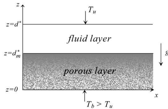
Figure 1. Geometric configuration of the problem.
