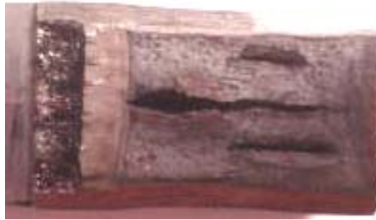
Figure 4. Typical fracture surface of shallow-cracked SE(T) specimen with main and secondary delaminations.
