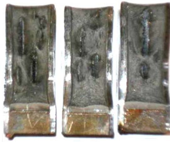
Figure 3. Typical fracture surface of shallow-cracked SE(T) specimens with multiple delaminations.
