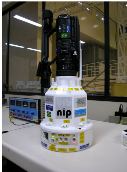
Figure 2. Experimental set up. The video camera mounted on the top chamber built with SLS technology.
