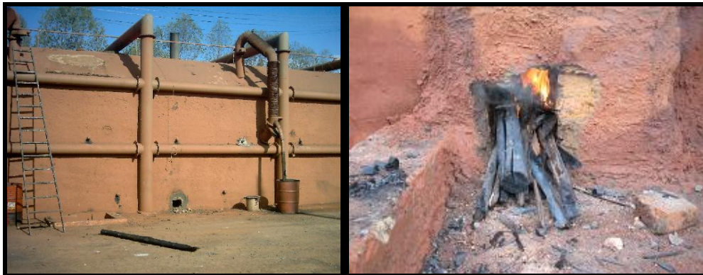
Figure 2. Ignition of the wood in a kiln FR-190 by a "tatu".
