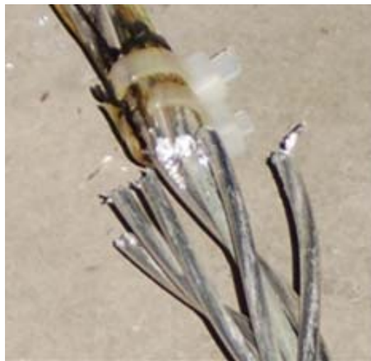
Figure 9. Test specimen after the 5 th wire cut
