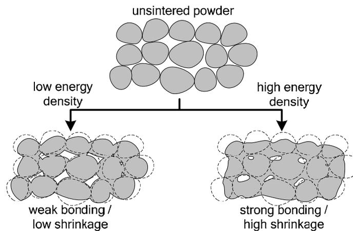
Figure 2. Bonding between the powder particles depending on the energy density.
