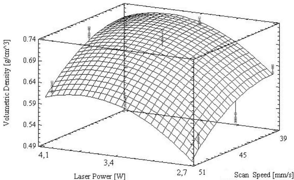
Figure 5. Estimated response surface for volumetric density.
