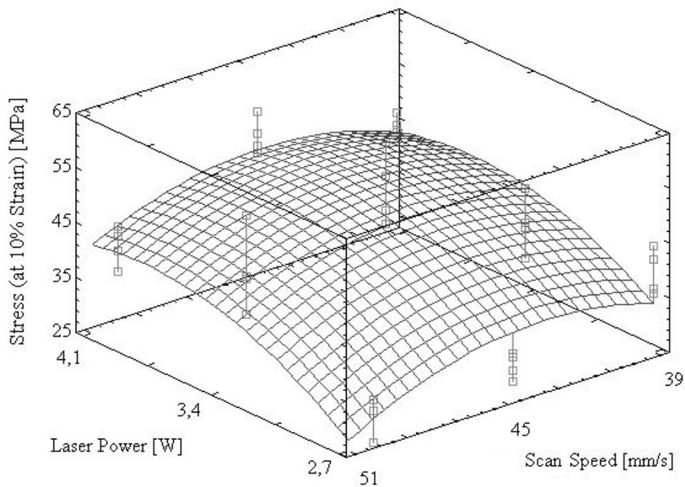
Figure 7. Estimated response surface for stress at 10% strain.
