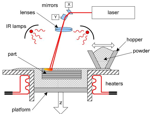
Figure 3. Schematic representation of the prototype SLS machine used in the experiments.
