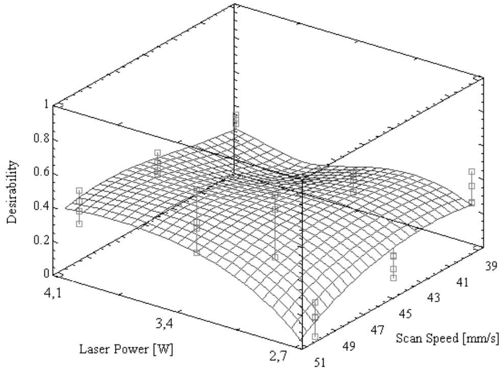
Figure 9. Estimated desirability surface for minimum density (porous material) with maximum stress and flexural modulus properties.
