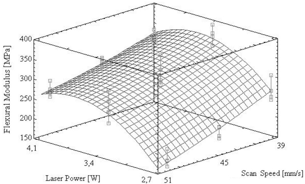
Figure 6. Estimated response surface for flexural modulus.
