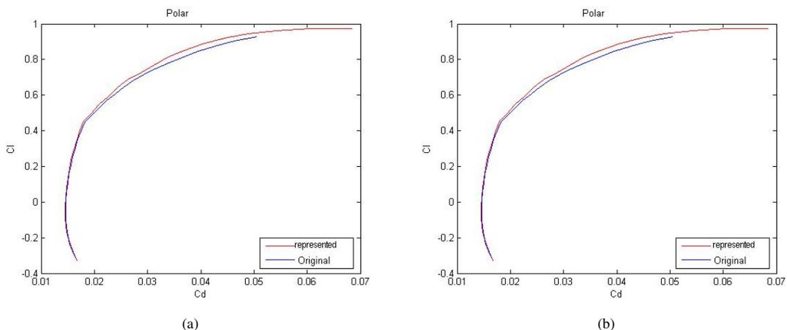
Figure 5. Polar convergence of NACA0012 for number of parameters a) 5BF; b) 7BF( $Re = 200.000$ )
