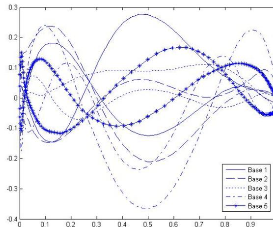
Figure 1. Set of 5 base functions derivate from the package of airfoils
