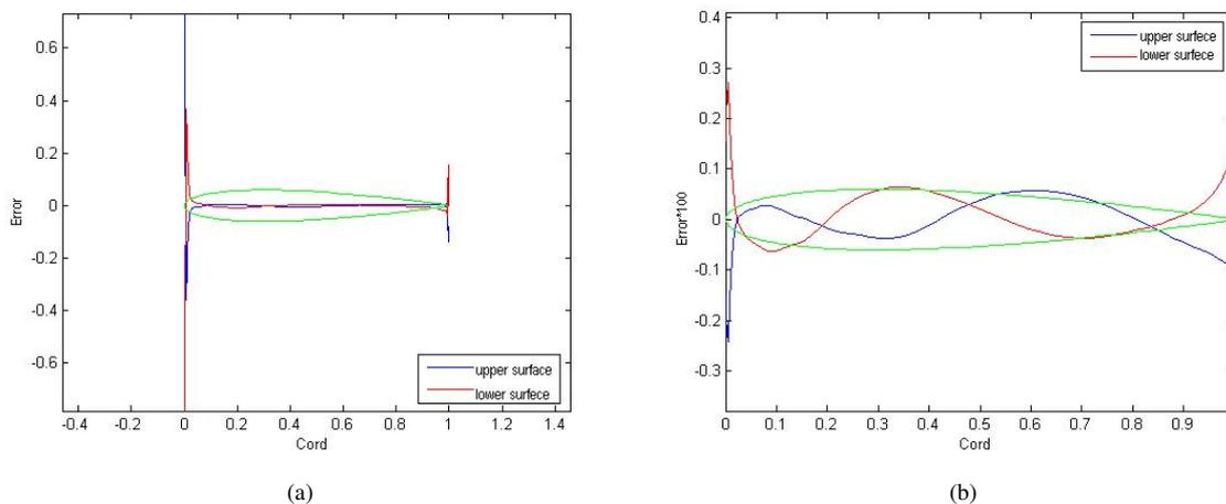
Figure 3. Geometric Errors a) 1<sup>st</sup> derivative e b) Thickness percent cord with 5 BF
