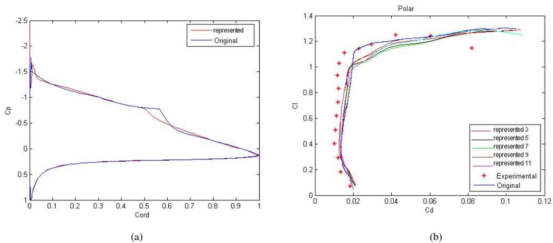
Figure 8. a) Eppler 387 Pressure distribution convergence with 7 BF ( $Re = 203.800$  e  $\alpha = 5^\circ$ ) b) Polar convergence of Eppler 387 ( $Re= 203.800$ )
