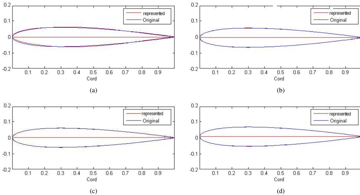
Figure 2. Geometric Comparisons for base functions a)3, b)5, c)7 e d)11
