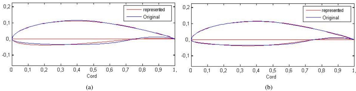
Figure 9. Geometric Comparisons for base functions a)3, b)7
