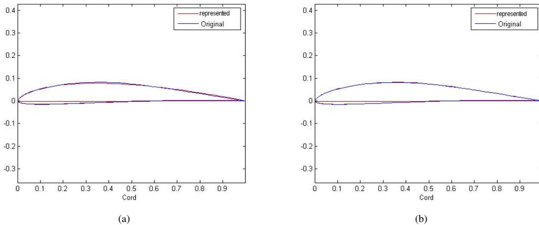
Figure 6. Geometric Comparisons for base functions a)3, b)5
