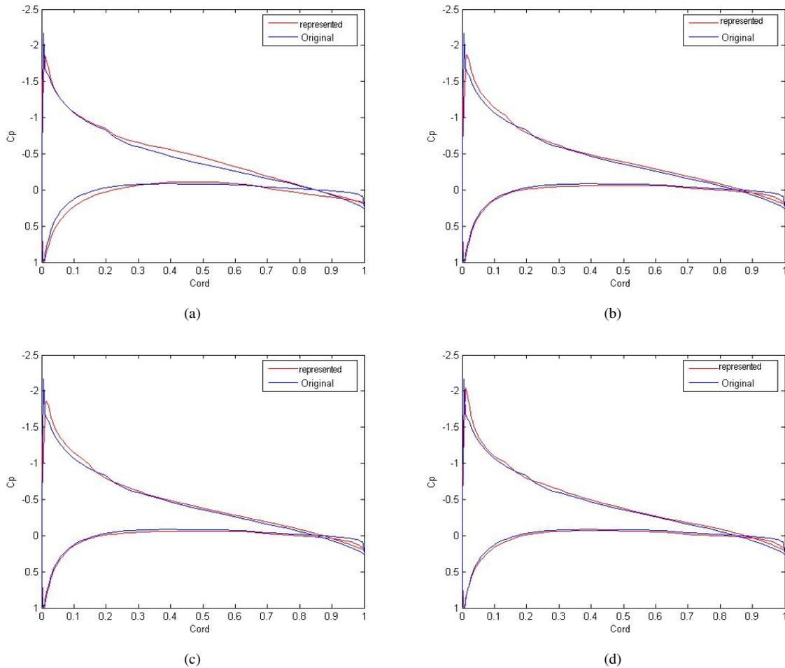
Figure 4. NACA0012 Pressure distribution convergence for a)3BF, b)5BF, c)7BF e d)11BF ( $\alpha = 5^\circ$ ,  $Re=200.000$ )
