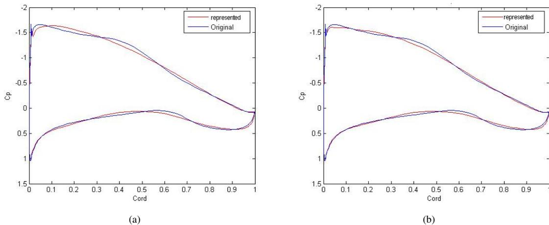
Figure 11. NFL (1) 0215f Pressure distribution convergence with a)9BF b)11BF ( $Re = 3.10^6$ ,  $\alpha = 0^\circ$  e  $M = 0, 4$ .)
