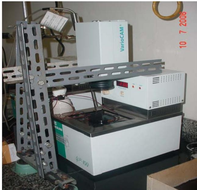
Figure 2 : Device for calibrating the thermographic camera at PUC-Rio
