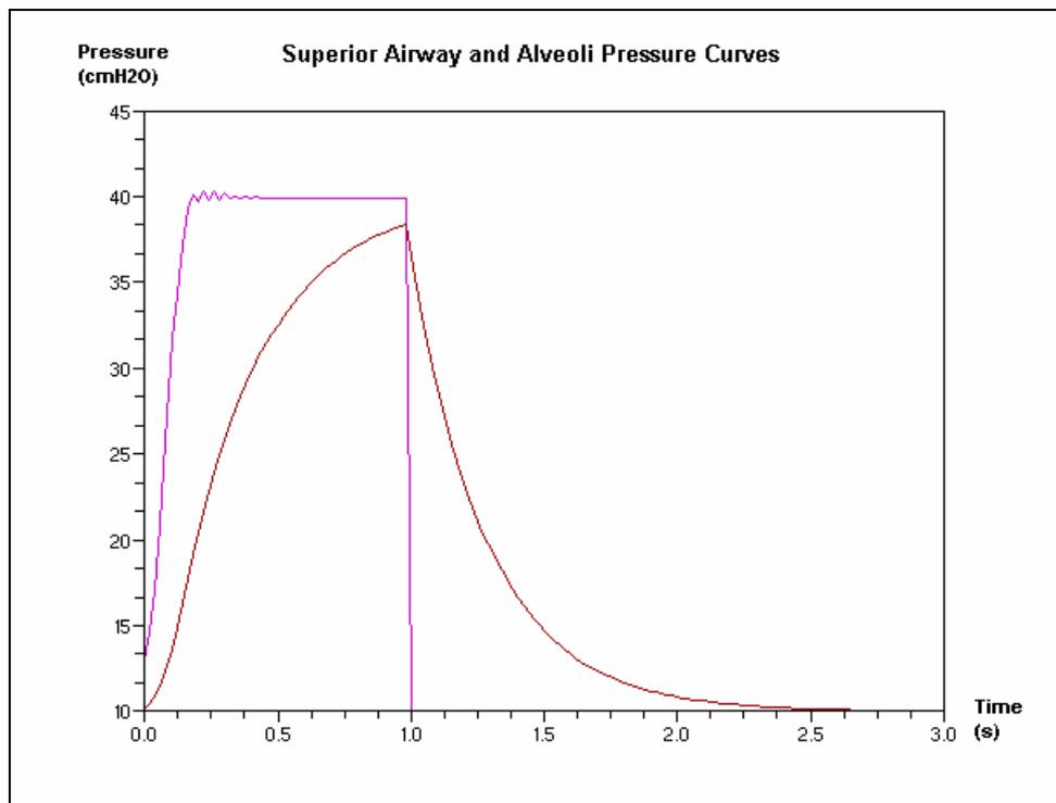
Figure 8. Case I. Pressure in the Superior Airway (red curve), in the Lung A ( $C_A=0.020L/cmH_2O$ , purple), in Lung B ( $C_B=0.010L/cmH_2O$ , coincident with lung A) with relative Fuzzy PID controller.
