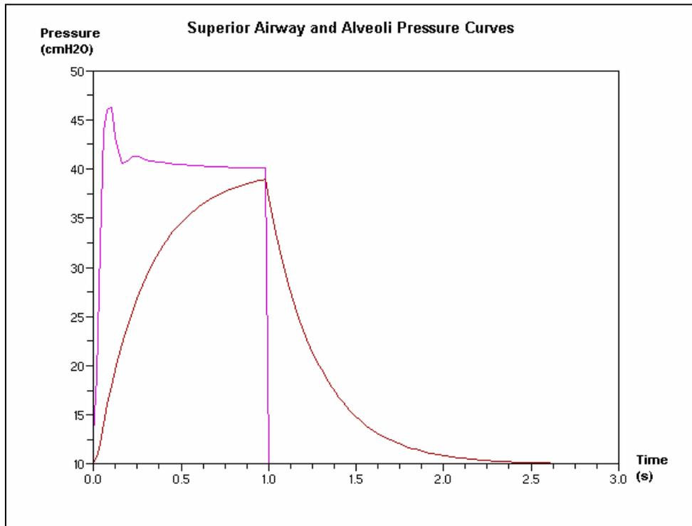
Figure 7. Case I. Pressure in the Superior Airway (purple curve), in the Lung A ( $C_A=0.020L/cmH_2O$ , red), in Lung B ( $C_B=0.010L/cmH_2O$ , coincident with lung A) with PID controller.
