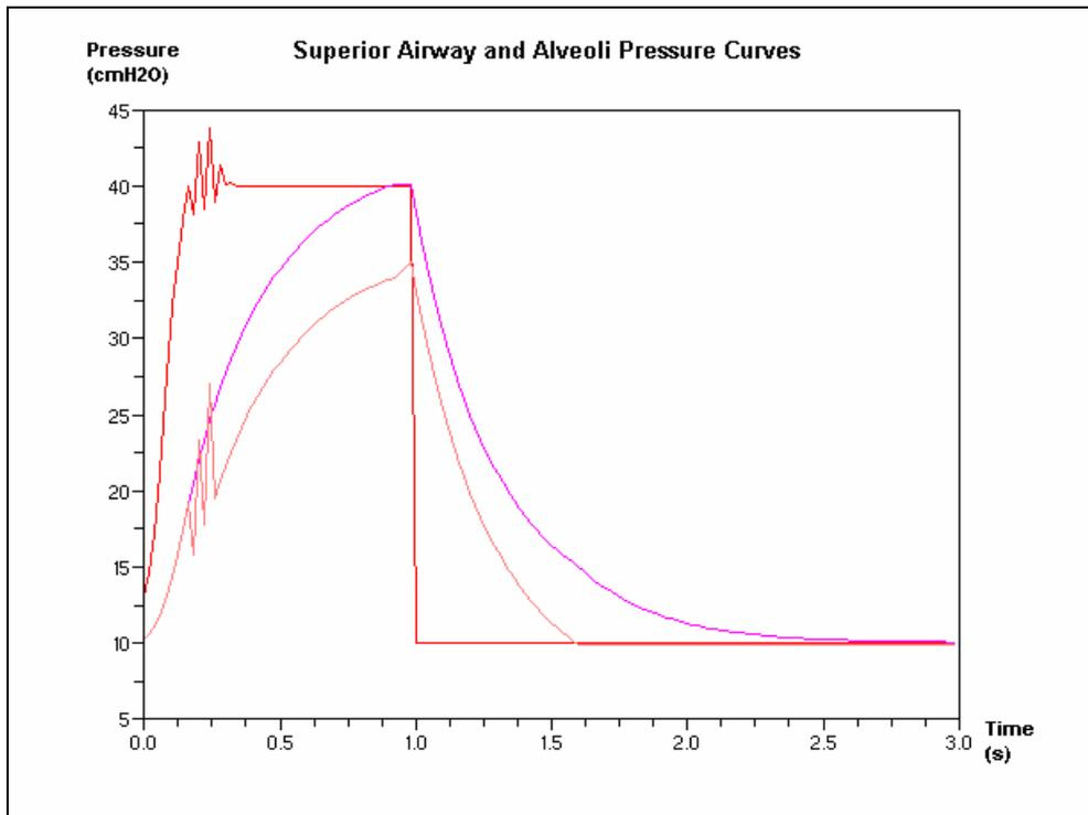
Figure 10. Case II. Pressure in the Superior Airway (red curve), in the Lung A ( $C_A=0.020\text{L}/\text{cmH}_2\text{O}$ , purple), in Lung B (variable  $C_B$ , light pink) with a relative Fuzzy PID controller.
