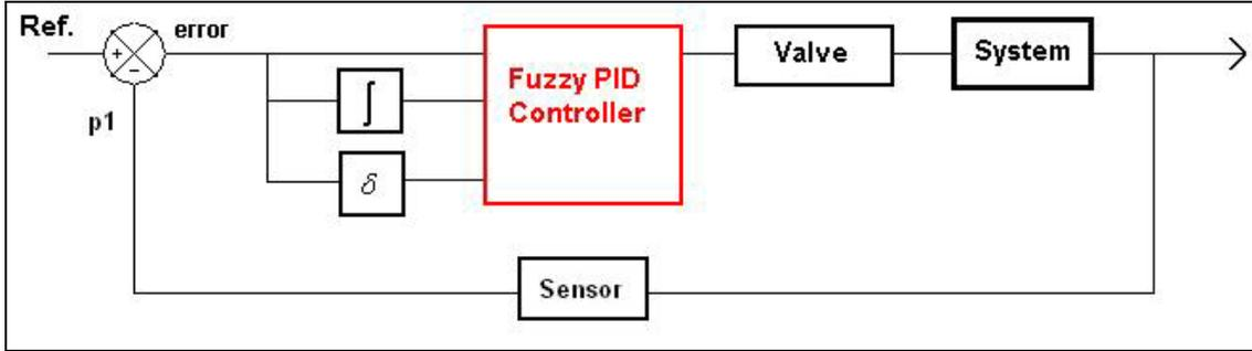
Figure 6. Block diagram of Relative PID Fuzzy Controller.
