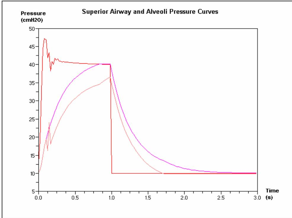
Figure 9. Case II. Pressure in the Superior Airway (red curve), in the Lung A ( $C_A=0.020\text{L}/\text{cmH}_2\text{O}$ , purple), in Lung B (variable  $C_B$ , light pink) with PID controller.
