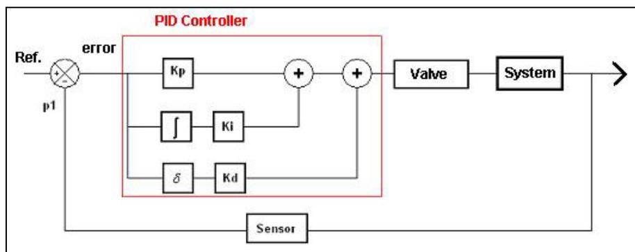
Figure 5. Block diagram of PID Controller.
