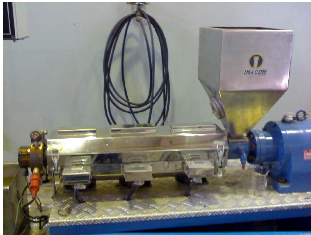
Figure 1- Extruder utilized in mixture of the materials (cellulose fibers/HDPE) composites.
