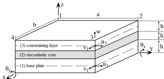
Figure 2. Illustration of the three-layer sandwich plate finite element.
