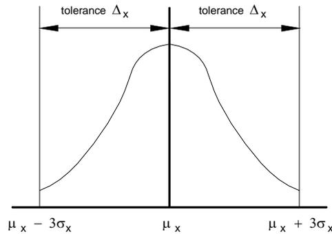
Figure 1. Mean standard deviation and the tolerance of design variables (Lee and Park, 2001).
