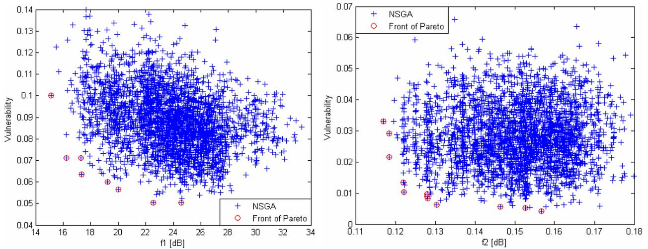
Figure 6 – NSGA solutions and the first front of Pareto for both objective and vulnerability functions
