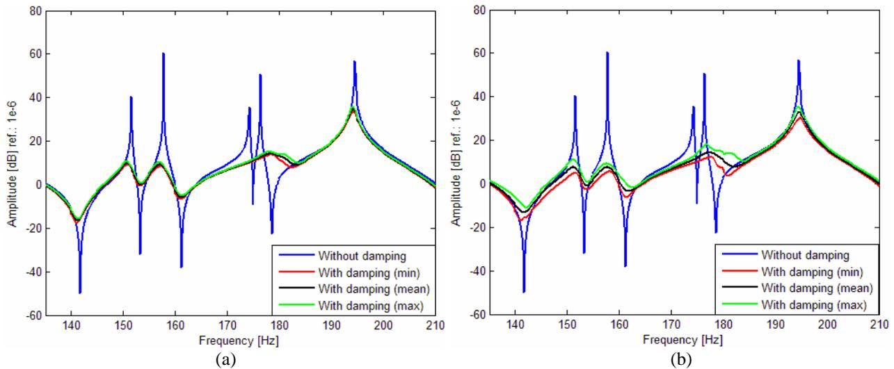
Figure 9 – Envelopes of dynamic responses for robust optimal solutions (a) and deterministic optimal solutions (b)
