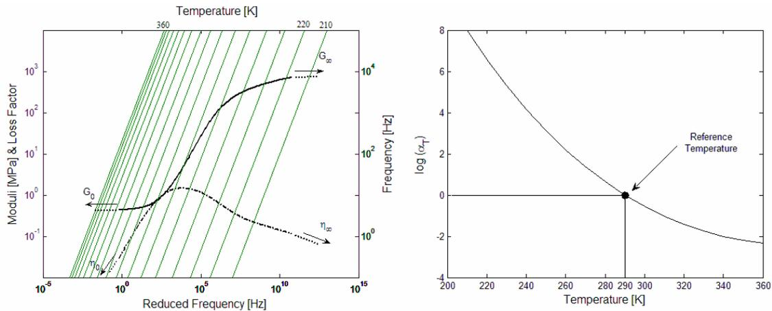
Figure 4 – Master (left) and shift factor curves (right) for the 3M ISD112™.
