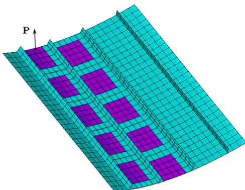
Figure 5. FE model of the stiffened panel treated with PCLD.
