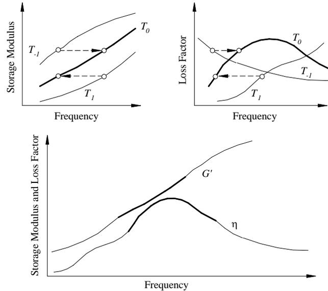
Figure 3 – Illustration of the frequency-temperature superposition principle
