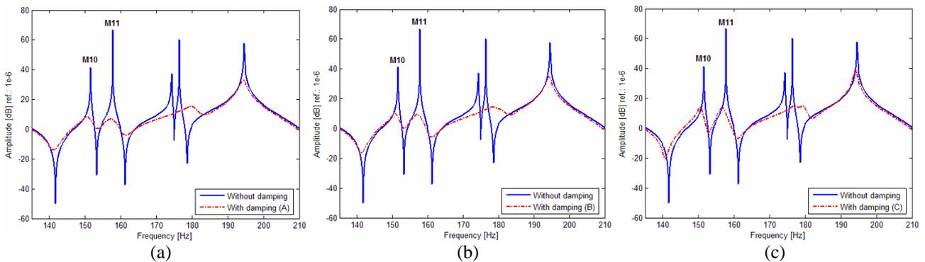
Figure 8 – Amplitudes of FRFs for the robust optimal design solutions **A** (a), **B** (b) and **C** (c)
