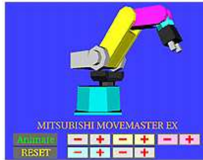
Figure 7. Interactive VRML interface for simplified robot programming
