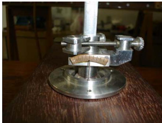
Figure 4. Mechanism used to allow the angle variation.
