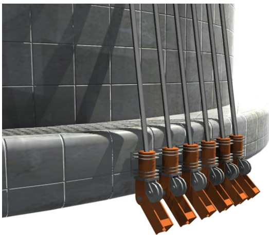
Figure 5. Image (a) shows a detail of the platform 3D model with its fair-leads. Image (b) is a deck model with the process plant that will be attached to the model.
