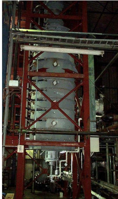
Figure 3. Dual-fuel burner with its oil gun.
