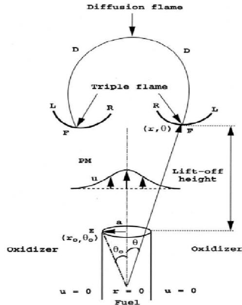
Figure 1. Schematic of the triple flame in a laminar lifted diffusion flame over a round jet (Ghosal and Vervisch, 2001).
