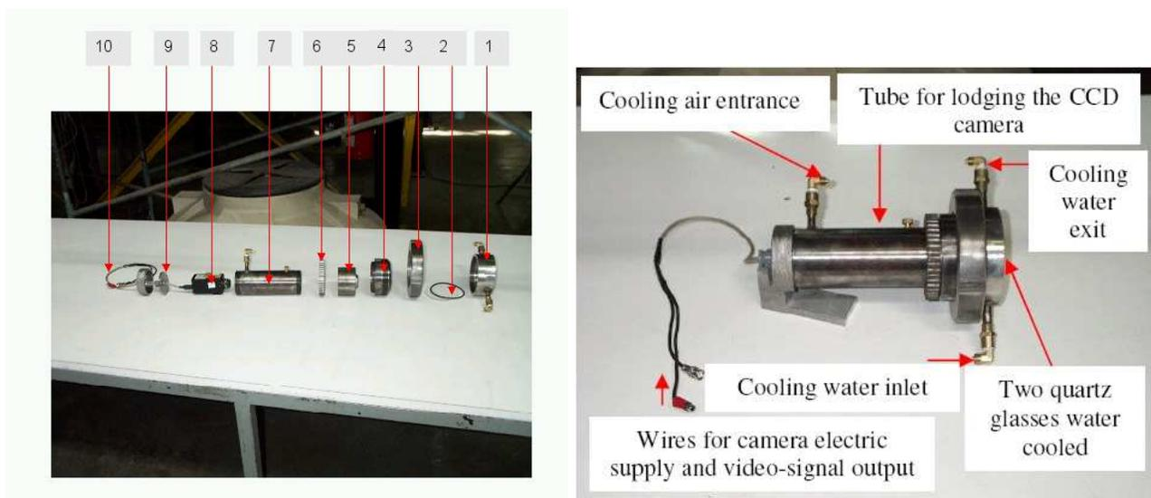
Figure 4. Exploded view of the optical set, 1) hatchway for lodging quartz glasses 2) quartz glasses and tightening ring 3) screw-nut for fixing the hatchway to the furnace wall 4) device for tightening the quartz glasses 5) device for lodging the interference filter 6) screw-nut for fixing the camera tube lodging to the hatchway 7) camera tube-lodging 8) *CCD* camera 9) optical set rear-closing device 10) wires for electrical camera supply and signal output.
