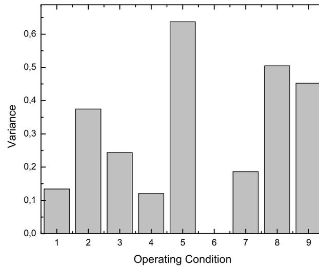
Figure 12. Variance values of the flame detector signal for all cases.
