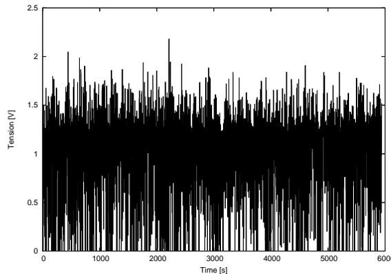
Figure 6. flame detector tension for the baseline operation condition - Case 1.
