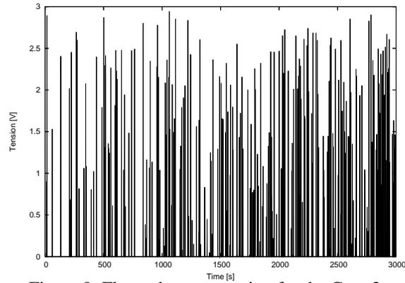
Figure 8. Flame detector tension for the Case 3.
