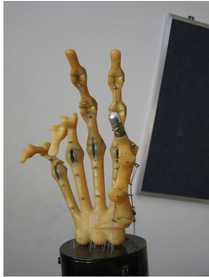
Figure 2. The mechanical structure of the Brazilian Anthropomorphic Hand (BRAHMA)
