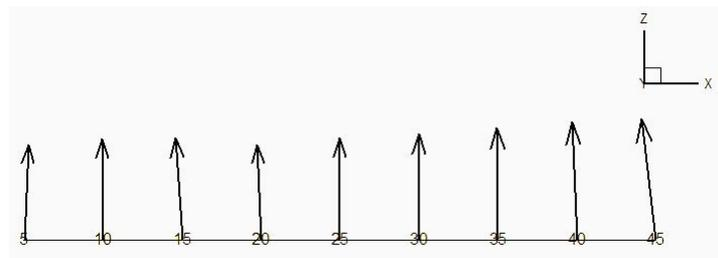
Figure 7. Velocity components in the horizontal plane of the swirling flow
