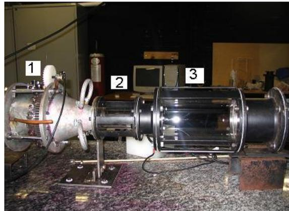
Figure 6. The LPP combustor. 1 - Swirler; 2 - Premixing chamber; 3 - Combustion chamber
