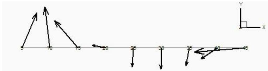
Figure 8. Velocity components in the transversal plane of the swirling flow
