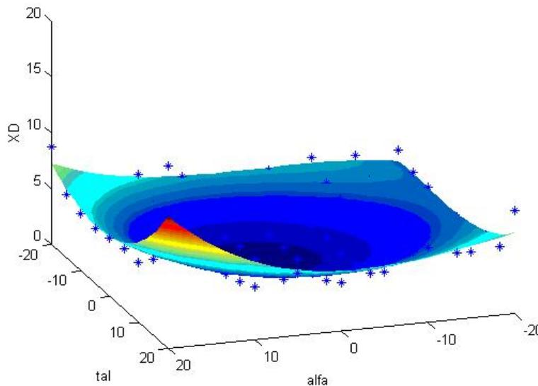
Figure 4. Dynamic pressure coefficient in function of yaw and pitch angles
