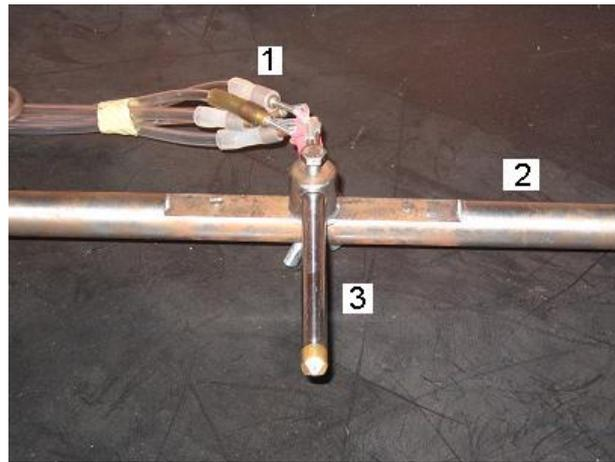
Figure 1. Five-Hole Pressure Probe 1 - Pressure Tap Outputs ; 2 - Horizontal axis; 3- The Probe.
