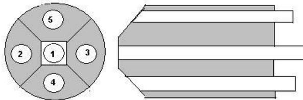
Figure 2. Five-Hole pressure probe; 1 - central pressure tap; 2 - 3 : pressure taps difference strongly affected by the yaw angle; 4 - 5: pressure taps difference strongly affected by the pitch angle
