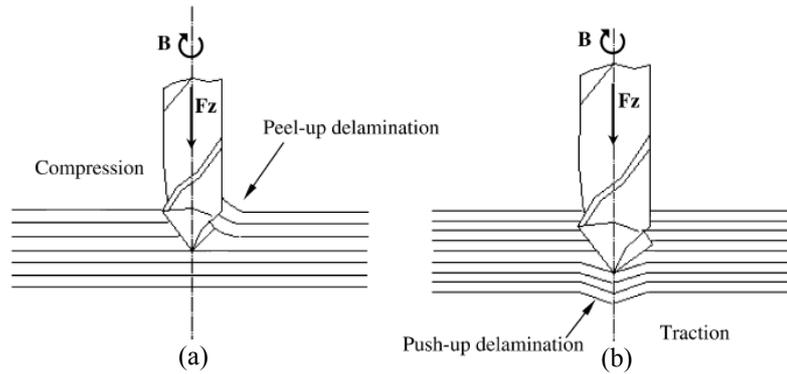
Figure 1. - Delamination at the tool entry (a) and exit (b) when drilling FRP laminate.
