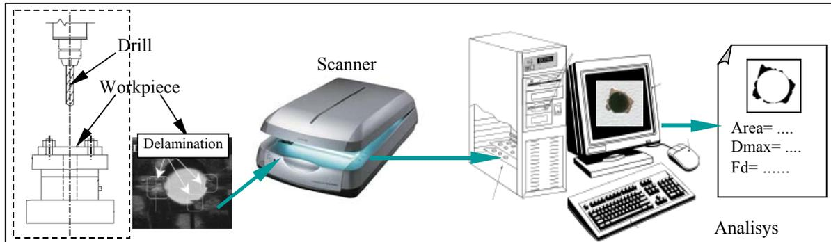
Figure 3. Acquisition system for measuring delamination.
