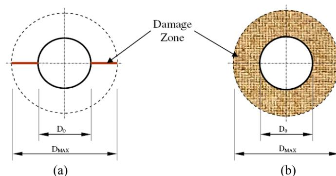
Figure 2 - Critical cases when drilling FRP laminate: (a) fine cracks and (b) uniform damage area.
