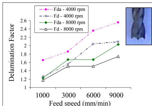
Figure 5 – The effect of feed speed on the conventional ( $F_d$ ) and adjusted ( $F_{da}$ ) delamination factors.
