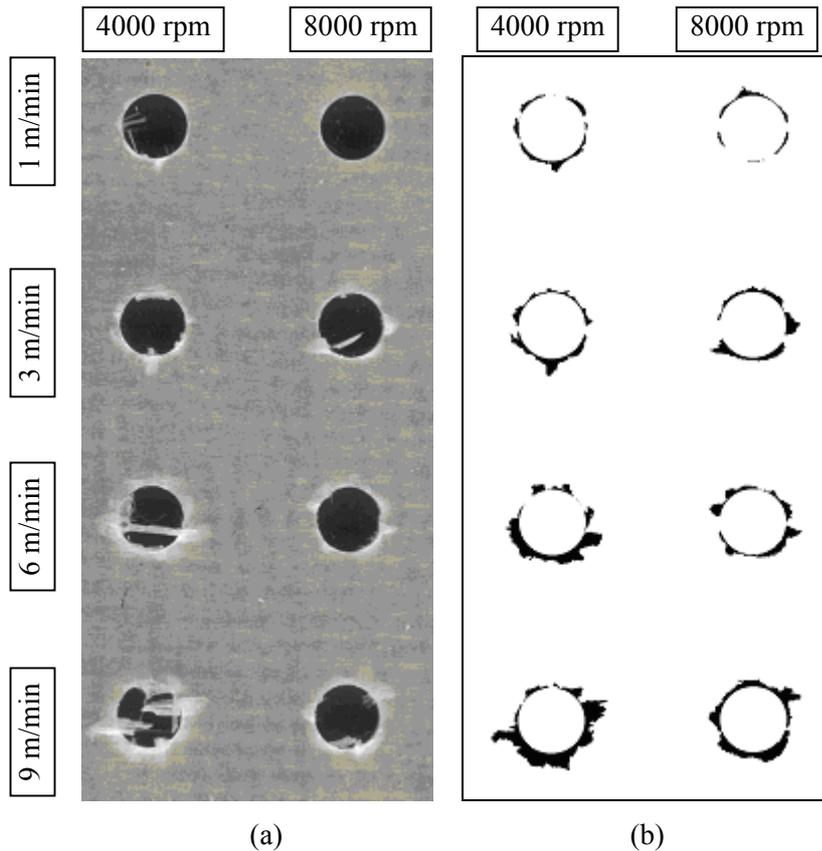
Figure 4 – Raw (a) and processed (b) images of the damage on glass fibre reinforced laminates.
