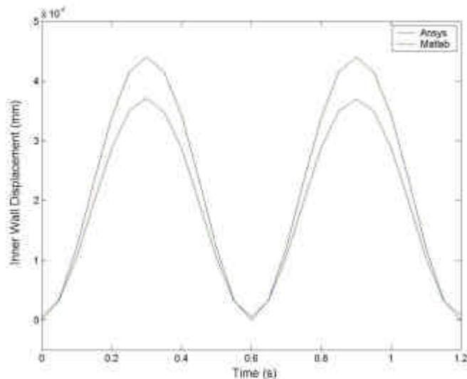
Figure 6 – Displacement calculated by ANSYS and MATLAB.
