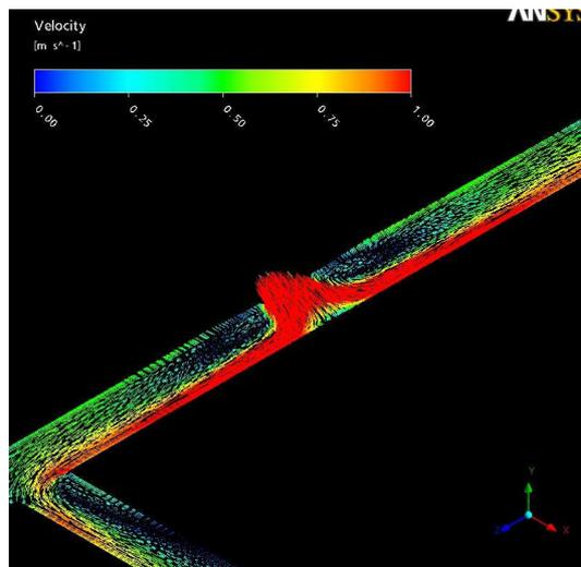
Figure 7 – Recirculation at the inlet tube end extremity
