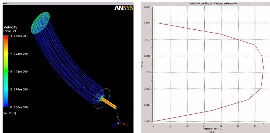
Figure 8 – Streamlines in the outlet tube 1 (left) and velocity profile (right) at the outlet tube back end.
