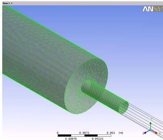
Figure 2 – Mesh along the tube and at the end of the outlet tube
