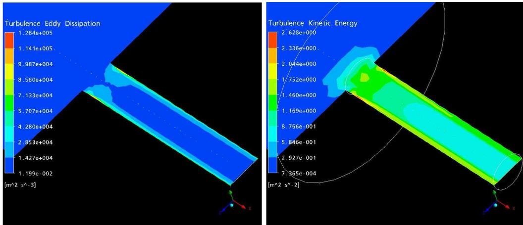
Figure 10 – Turbulent eddy dissipation and turbulence kinetic energy along the outlet tube back end.
