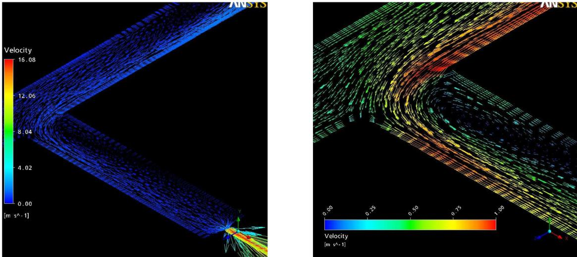
Figure 6 – Vortex at the second tube and a detailed view of the recirculation.
