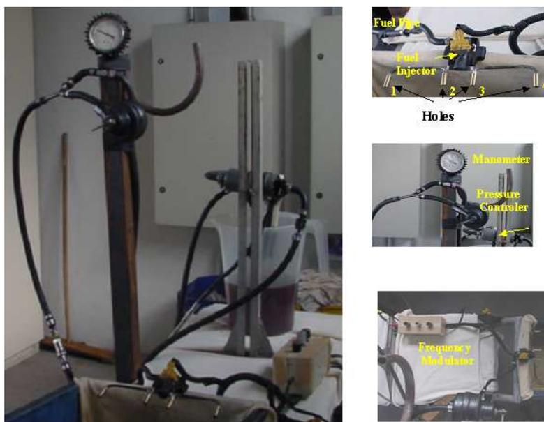
Figure 3. Overview of experimental setup.
