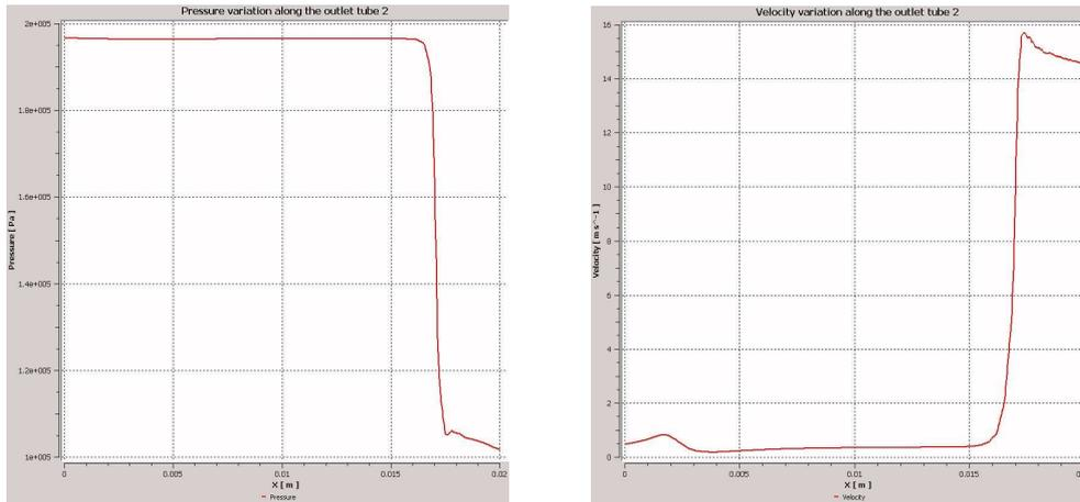
Figure 7 – Pressure (left) and velocity (right) variation along the outlet tube centerline.
