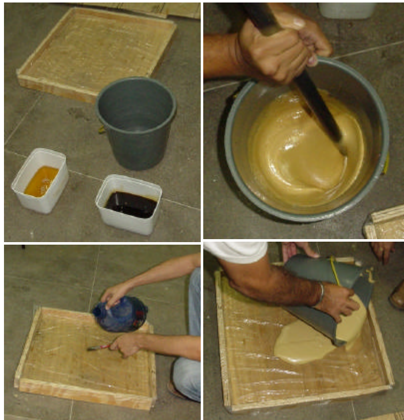
Figure 4 – Stages of COF plate fabrication process
