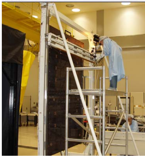
Figure 6: CBERS-2B EPSA panel final acceptance visual inspection performed at LIT/INPE.
