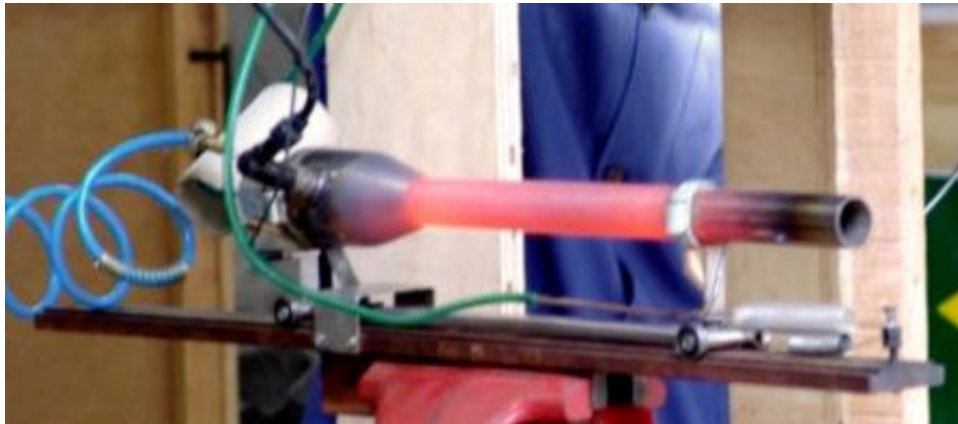
Figure 2. Pulse jet steady state operation
