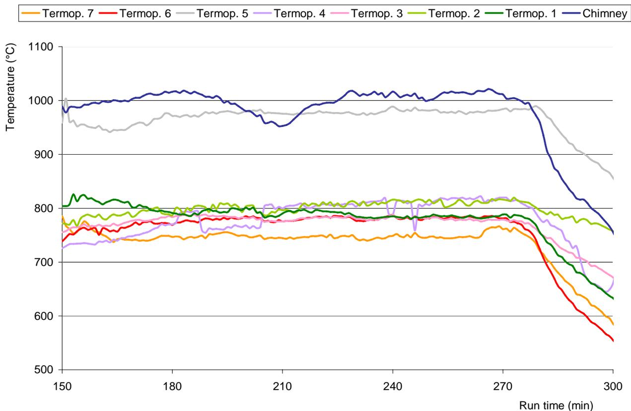
Figure 4: Gases temperature behavior, with time, for the gases at the furnace wall at all eight ports
