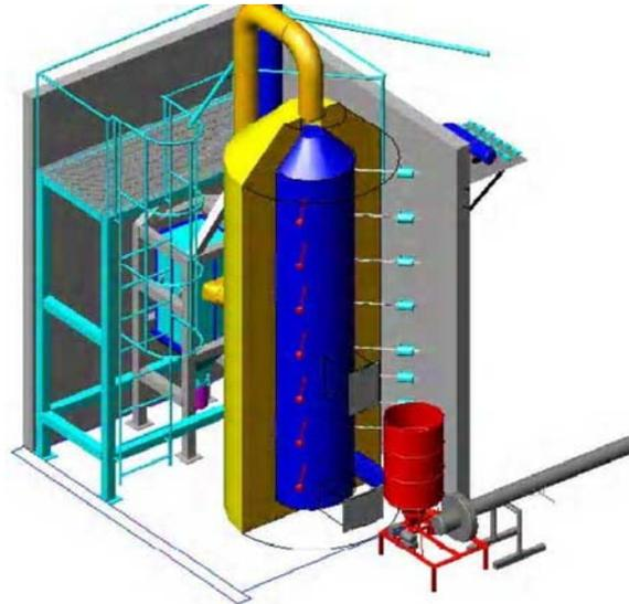
Figure 1: The cyclone furnace built at EBMA/UFPA facility
