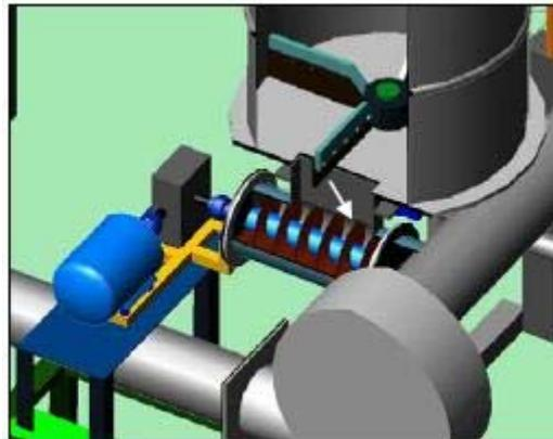
Figure 2: Air-sawdust geeding system
