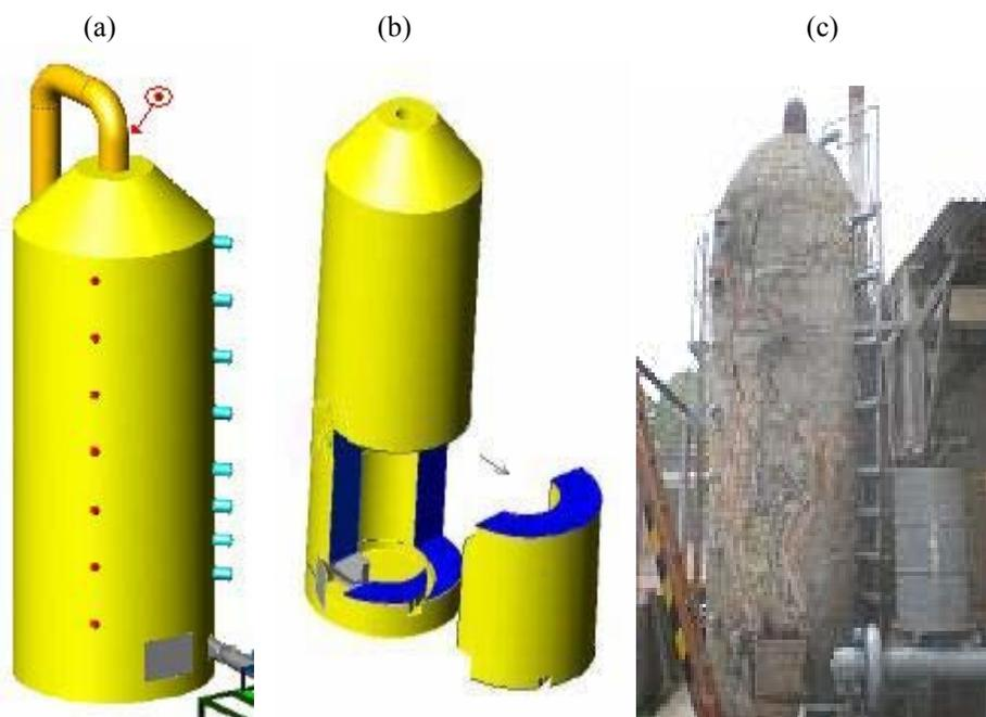
Figure 3 : (a) cyclone combustor external view ; (b) exploded view ; (c) picture of constructed combustor
