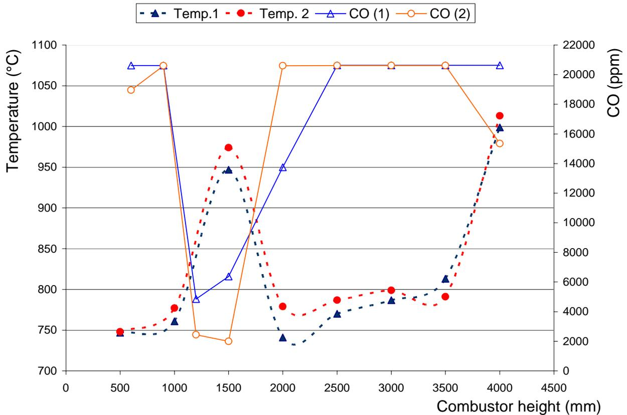
Figure 5: Temperature and CO profile, at furnace wall and furnace exit. (1) is for equivalence ratio of 0.78 and (2) for equivalence ratio of 0.83.
