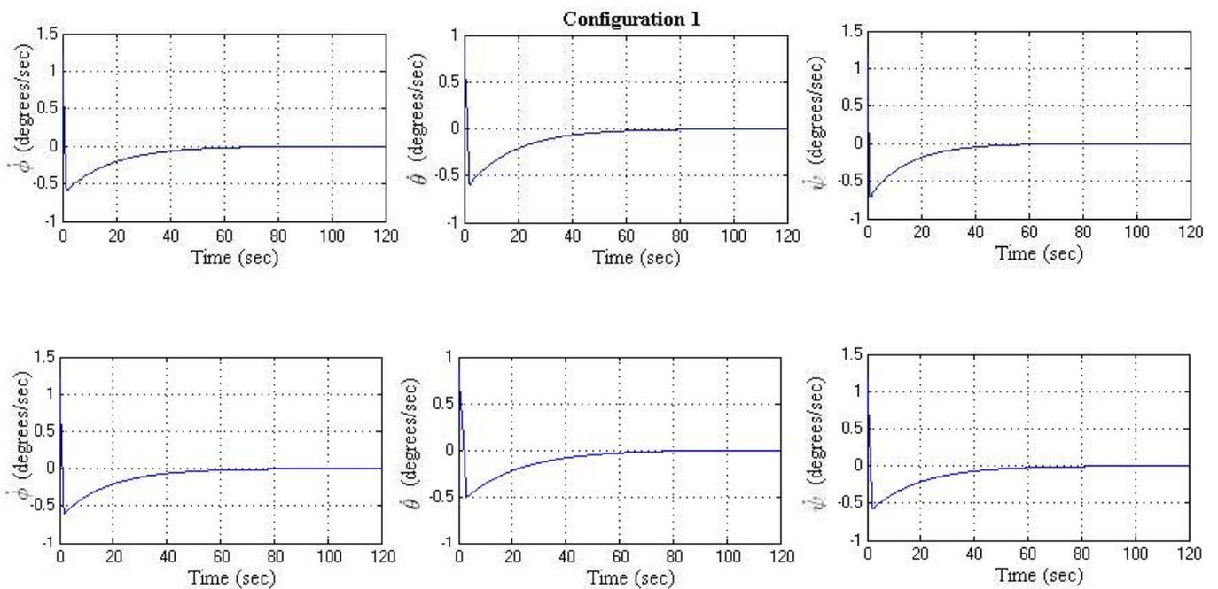
Figure 4. The Euler angle rates during the simulated maneuver.
