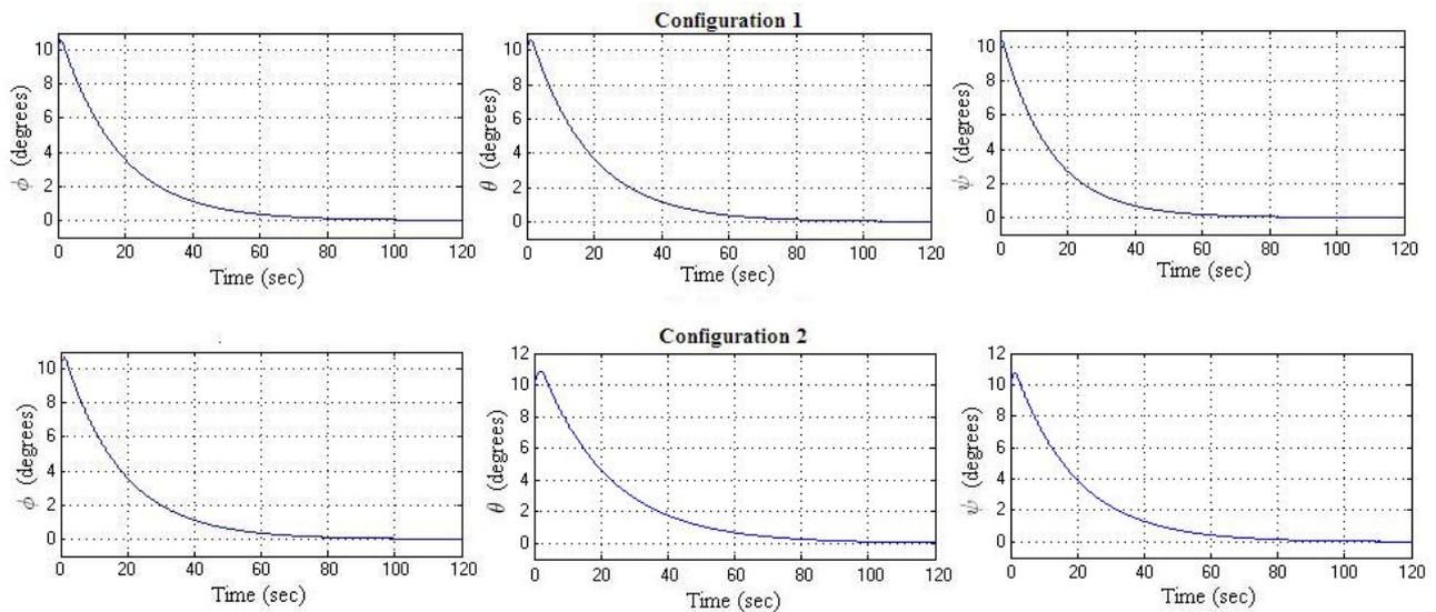
Figure 3. The attitude angles evolution during the simulated maneuver.
