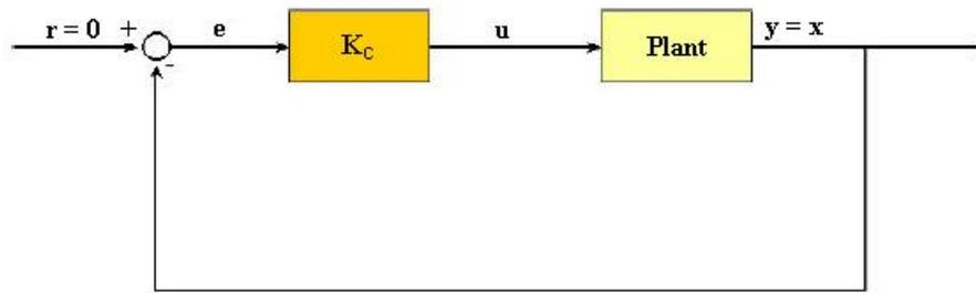
Figure 2. The block diagram of the LQR controller.
