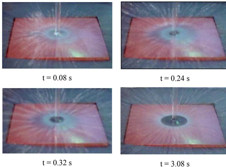
Figure 3: Photographs of the plate for the 3.08 s of the cooling process, water at  $26^\circ\text{C}$  and  $6 \text{ ℓ/min}$ .
