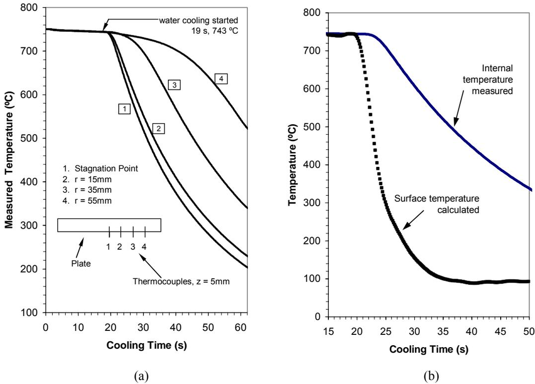
Figure 4: (a) Measured internal temperatures for  $3$  l/min and  $12^\circ\text{C}$  at  $r$  positions the radial distance from centre of the plate; (b) Calculated surface temperature and measured internal temperature, at  $r = 15$  mm and  $z = 5$  mm from stagnation point for  $3$  l/min and  $12^\circ\text{C}$ .
