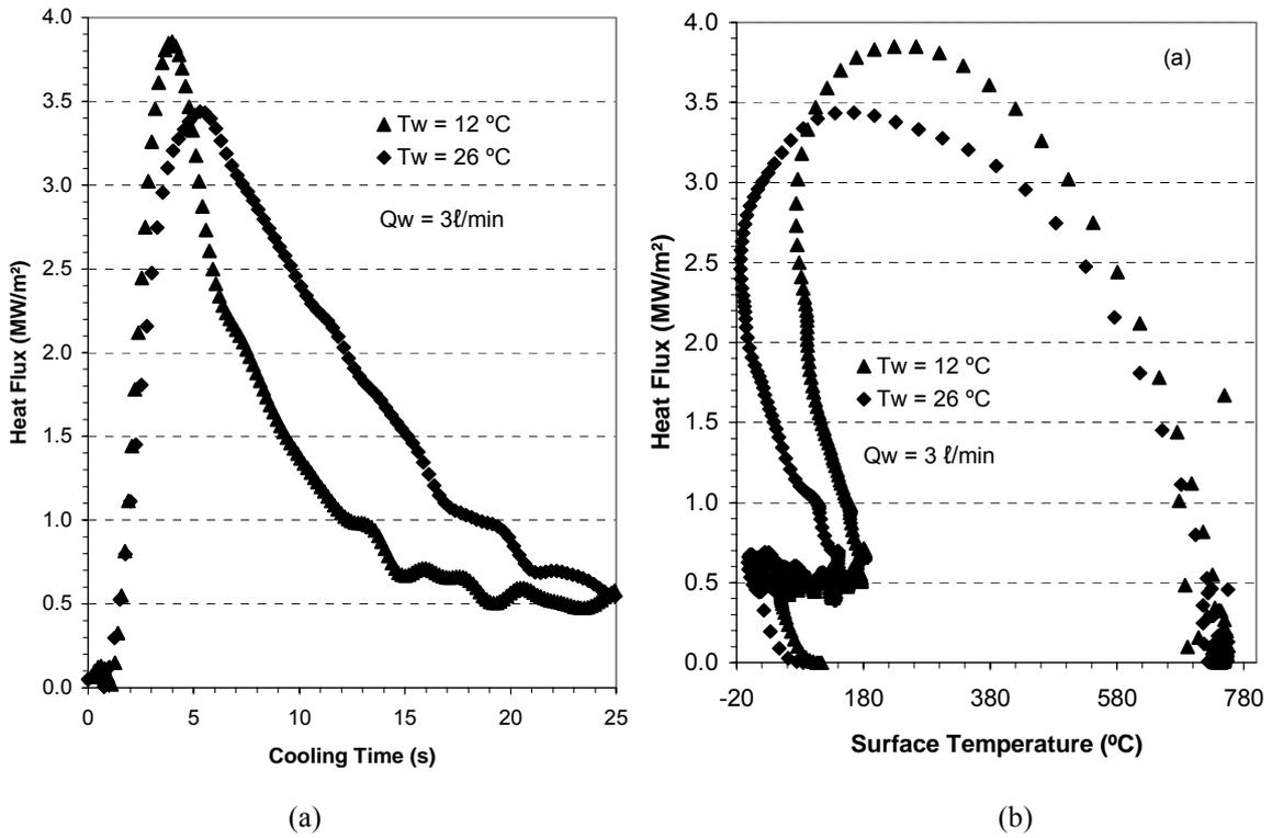
Figure 7: Effect of the water temperature. (a) Partial boiling curve; (b) Surface heat flux history.
