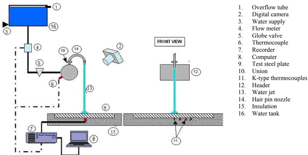
Figure 2: Outline of the experimental apparatus
