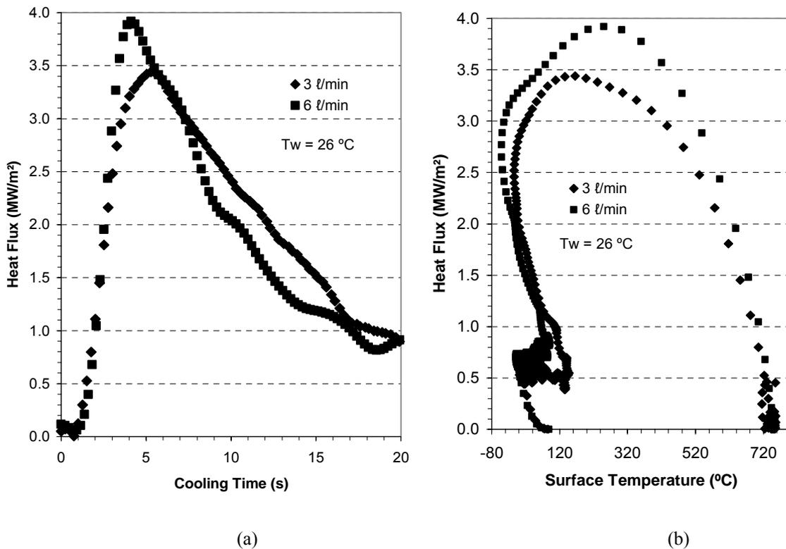
Figure 8: Effect of the flow rate, at  $r=0$ , with  $T_w=26^\circ\text{C}$ . (a) Partial boiling curve; (b) Surface heat flux history.
