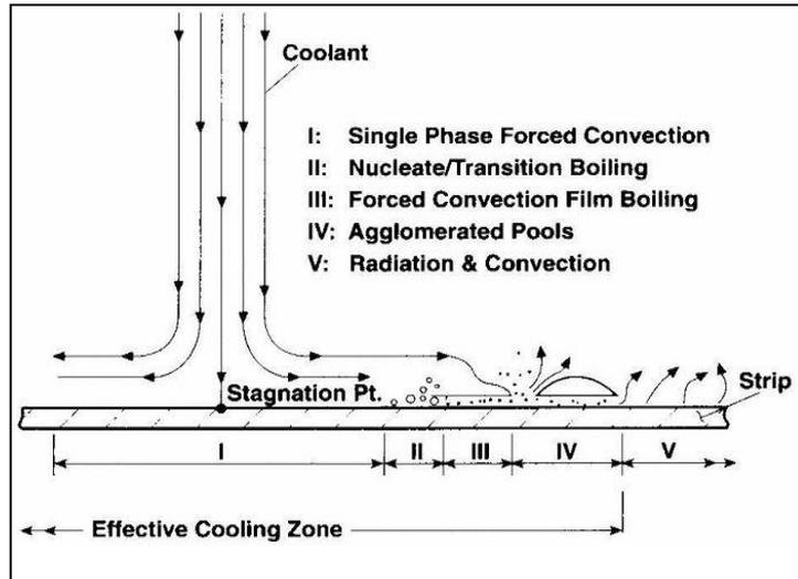
Figure 1: Heat transfer regimes adjacent to a jet impinging on hot strip (Zumbrumen *et al*, 1989).
