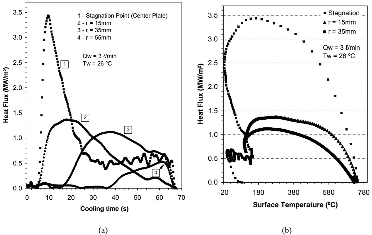
Figure 6: (a) Surface heat fluxes at given locations as function of time; (b) Boiling curves as function of surface temperature for  $r=0$ , 15 mm and 35 mm.
