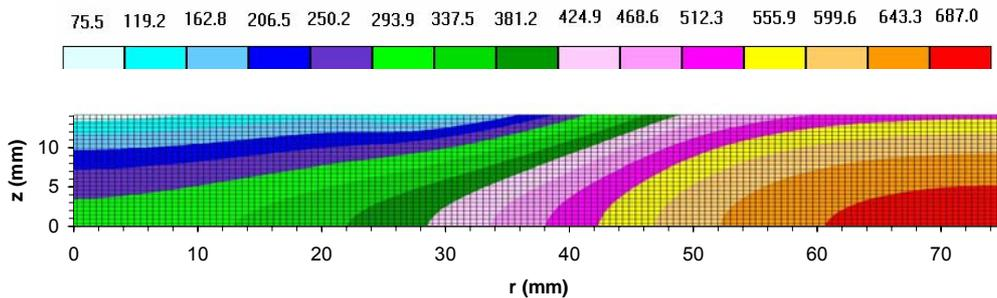
Figure 5: Isothermals at 25 s after start cooling process for  $3$  l/min and  $12^\circ\text{C}$
