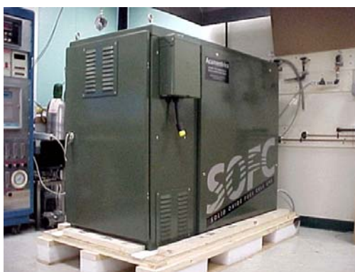
Figure 5 - SOFC (5kWe) system from Acumentrics.
