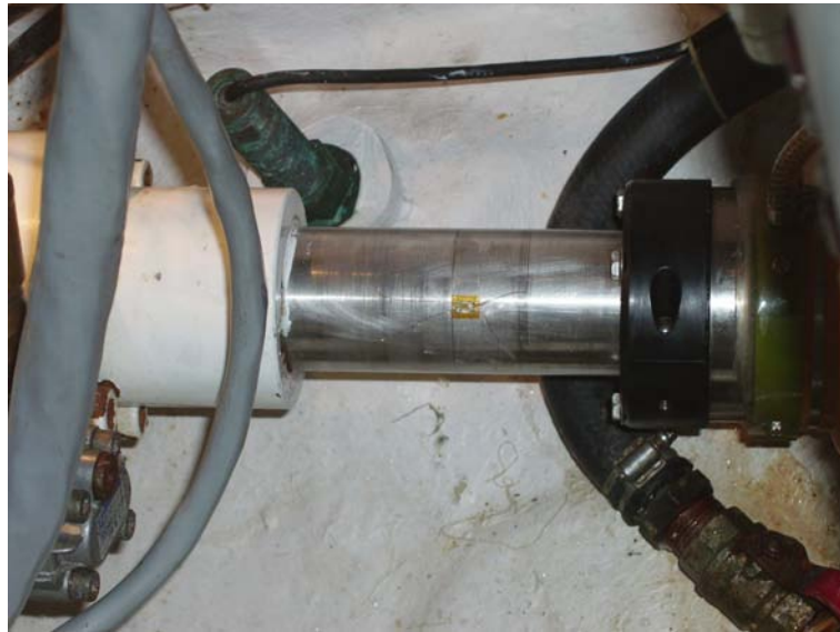
Figure 1. Strain gage applied to output shaft
