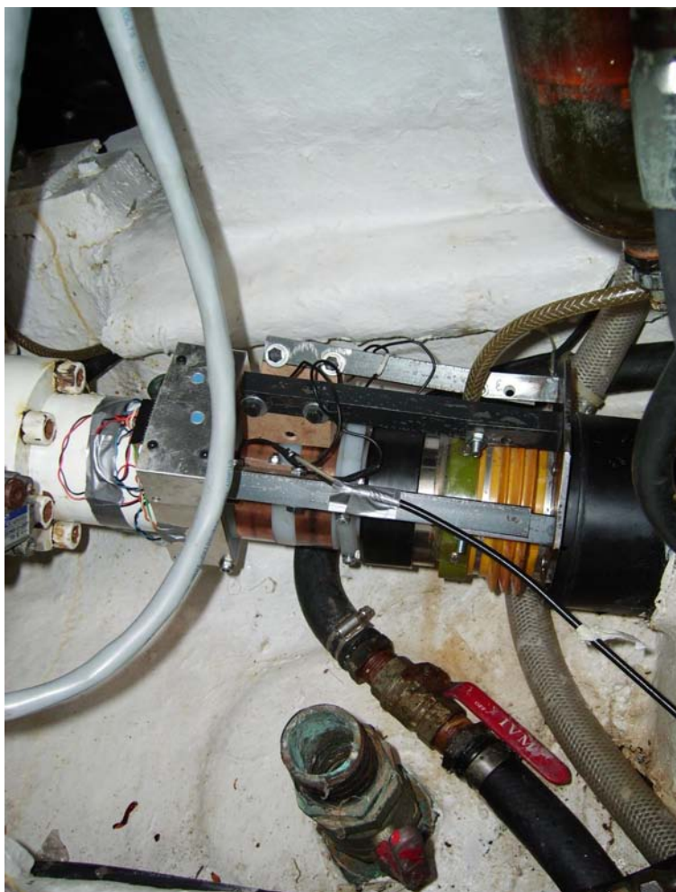
Figure 7. Slip-Ring assembly in engine output shaft
