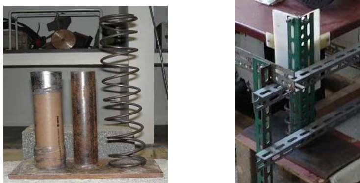
Figure 2 . Details of the spring and platform guides
