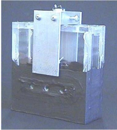
Figure 4: Heater tank and Agitator.
