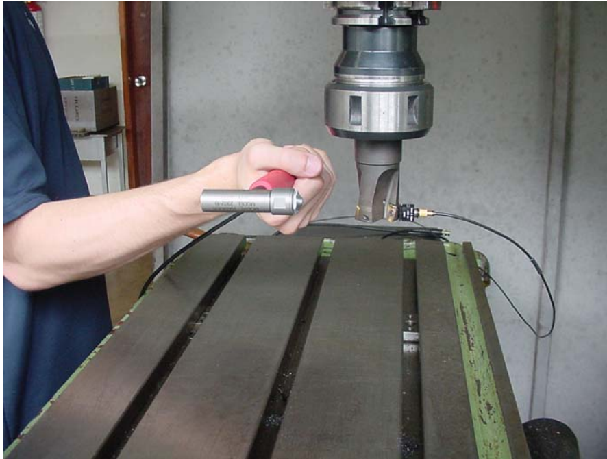
Figure 7 - Impact applied at the tool tip.
