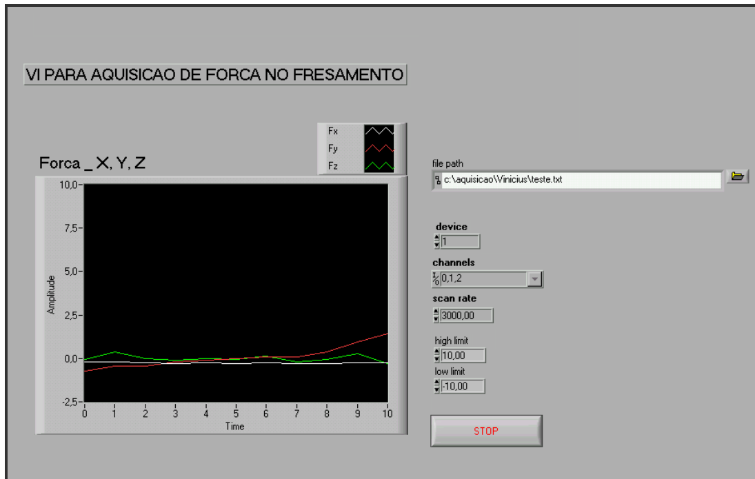
Figure 5 - LabView® virtual instrument. Translation: “Virtual instrument for milling forces acquisition”.
