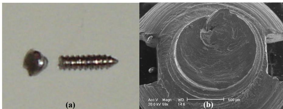
Figure 6. (a) tested titanium screw (b) SEM fractography of upper portion of a tested titanium screw.
