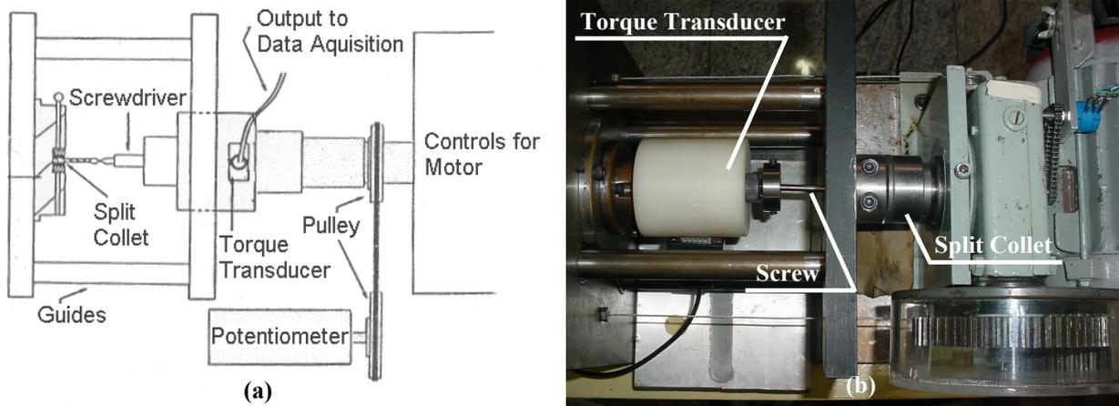
Figure 3. (a) Apparatus according ASTM F 543-02; (b) developed equipment .
