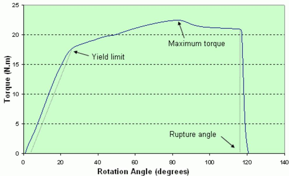
Figure 4. Typical result for breaking angle and maximum torque tests.
