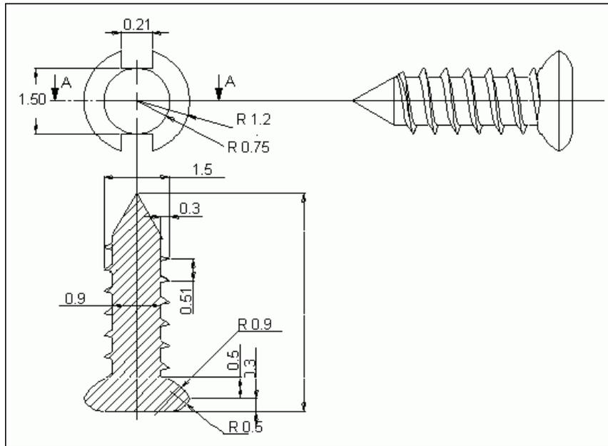
Figure 1. Titanium screw profile and dimensions.
