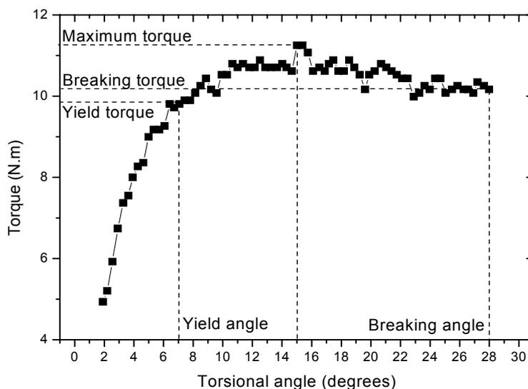
Figure 5. Result for torque versus angular displacement for titanium screw.
