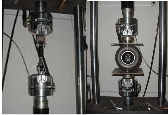
Figure 3. Experimental trial to determine the stiffness parameters of spring and tire, respectively.
