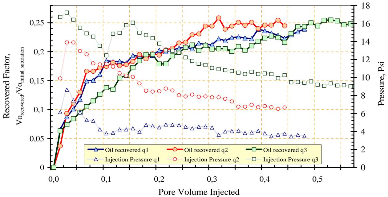
Figure 3. Oil recovered fraction, by three water injection flow rates  $q_1$ ,  $q_2$  and  $q_3$ , and their injection pressures.
