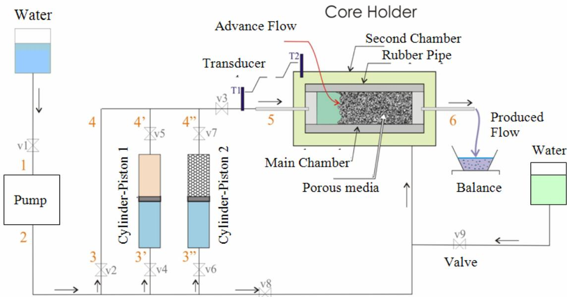
Figure 1. Schematic representation of experimental setup, (i) 3-4 when water is injected, (ii) 3'-4' when oil is injected, and (iii) 3''-4'' when emulsion is injected.
