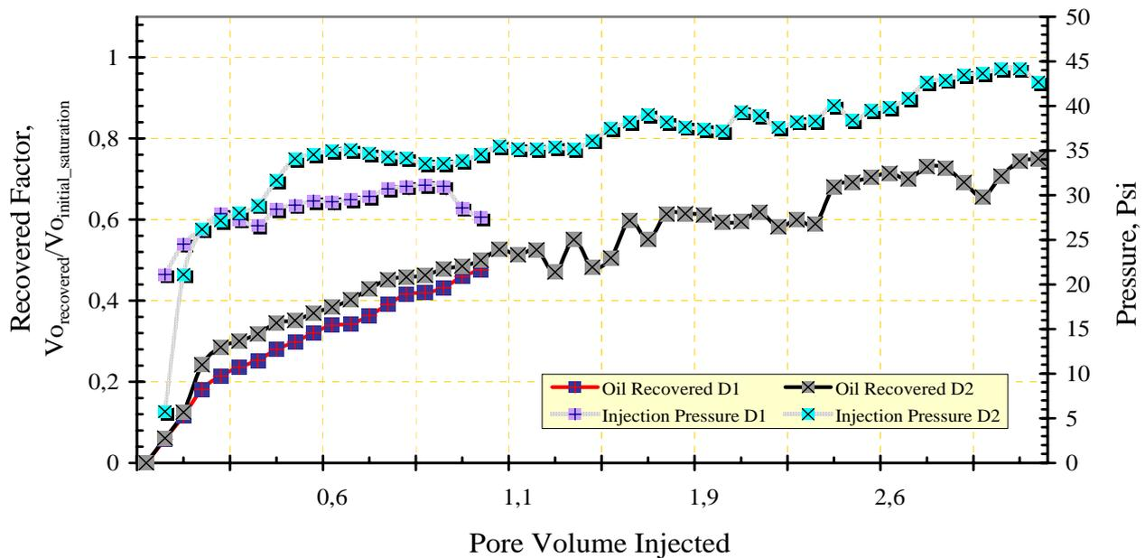
Figure 4. Oil recovered fraction, by emulsion injection of average drops D1 & D2, and their injection pressure.
