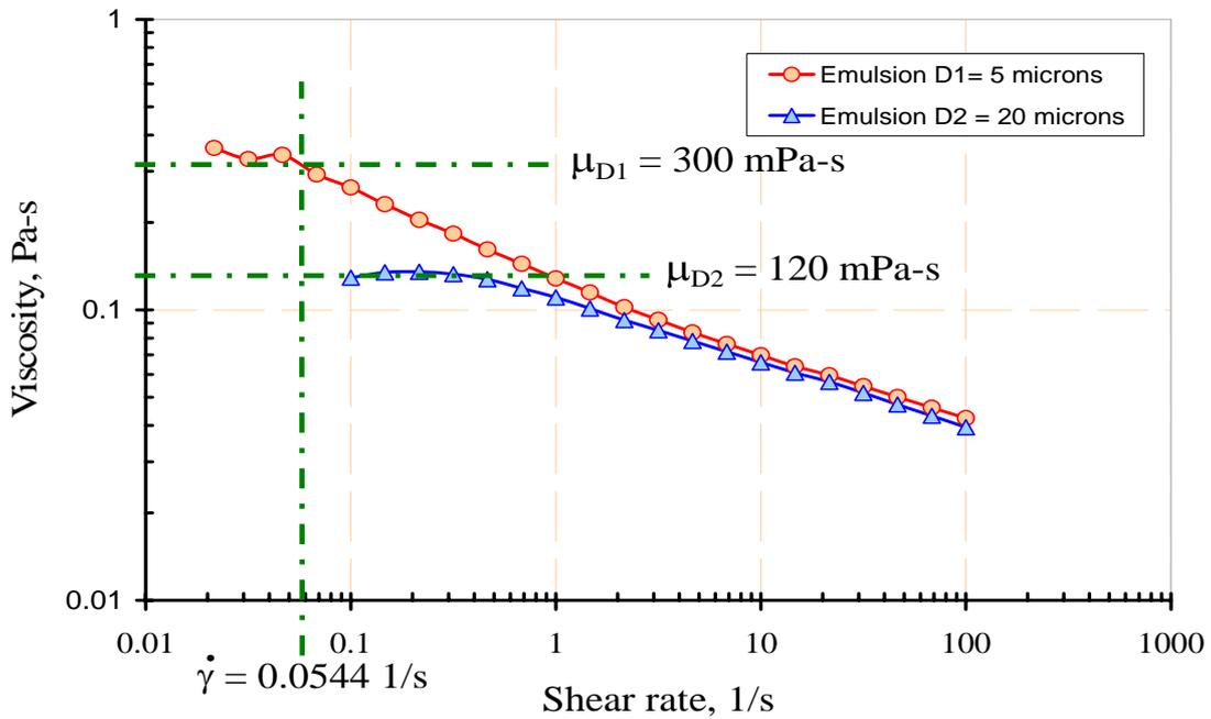
Figure 2. Variation of the viscosity with respect to the shear rate for the two emulsions:
