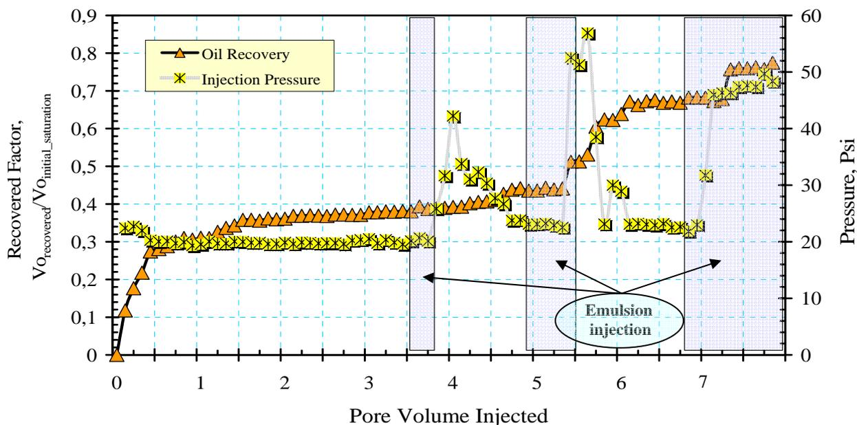
Figure 5. Results of oil recovered fraction, by alternate water and oil-water emulsion injection of average drop diameter  $D_2$ , and their respective results of injection pressure.
