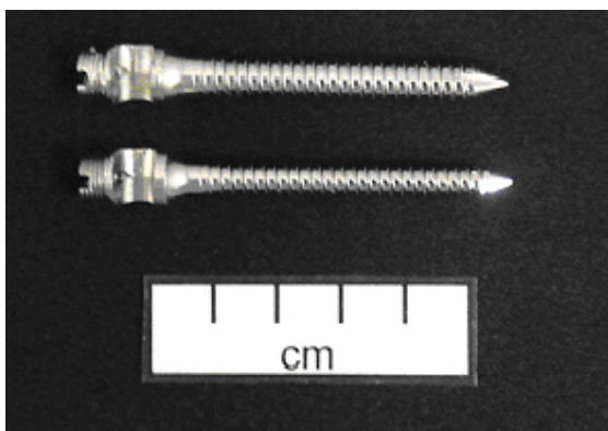
Figure 1 - Pedicular screw with external diameter of 5 and 6 mm.
