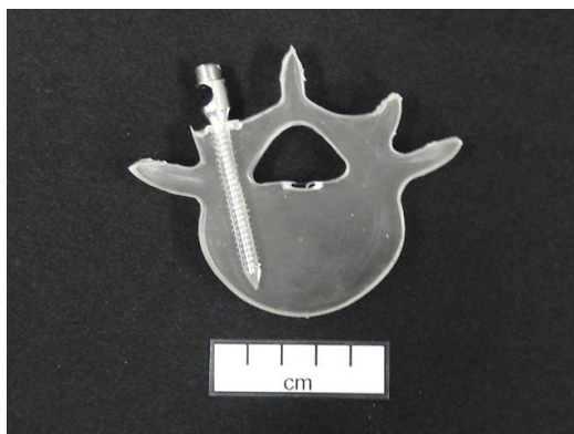
Figure 2 - Screw orientation inside the vertebrae.
